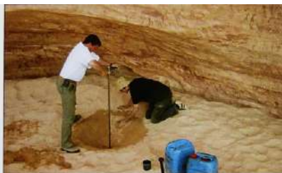
Fig. 10 Oliver Palm and Jan Kuper coring to assess the depth of the sand in the shelter.
